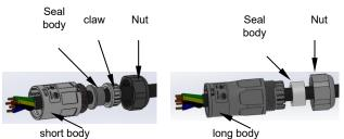
b Crimp wires screw twisting torque 0.8+/-0.1N·m
